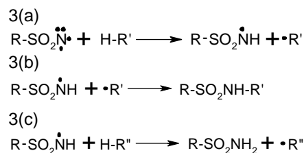
Scheme 3. Reaction of triplet nitrene with hydrocarbon. (a) Formation of macroradical by abstraction. (b) Formation of secondary sulfonyl amide by recombination. (c) Formation of primary sulfonyl amide by abstraction of a second proton.
